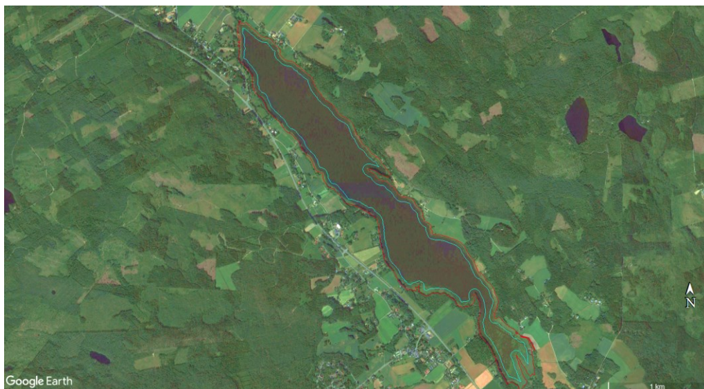
Figure 42 An example of a negative buffer of 50m shown in light blue line and original jarvi-10 area in red, applied for lake Suolijärvi. A vast majority of shoreline vegetation has been removed from the internal buffered area except for the south-eastern end of the lake. Base map view using Google Earth.
