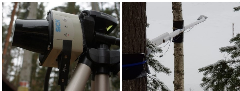
Figure 34 Left: laser scanner before installation; right: after installation above the lake using a wooden pole.
