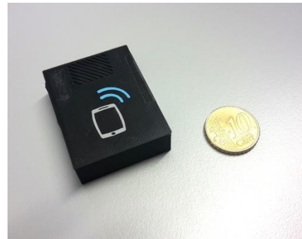
Figure 8. Telocate's ultrasound emitter compared to a 10 cent coin.
