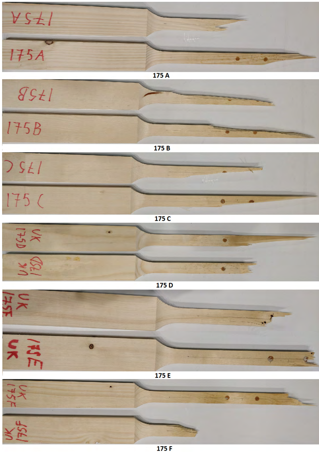
Figure D.6: Breakage of samples at 175 °C
