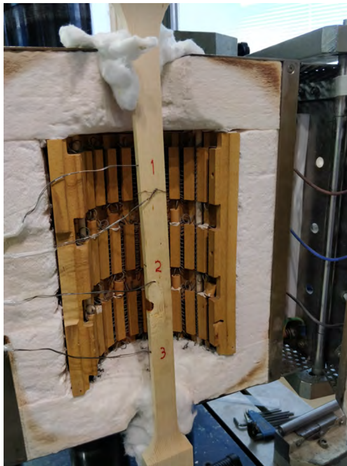
Figure 3.5: Thermocouples placed within the sample
