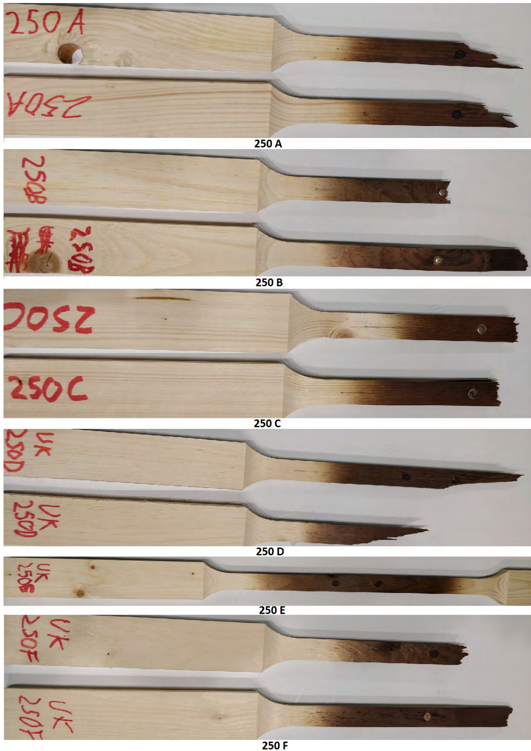
Figure D.9: Breakage of samples at 250 °C
