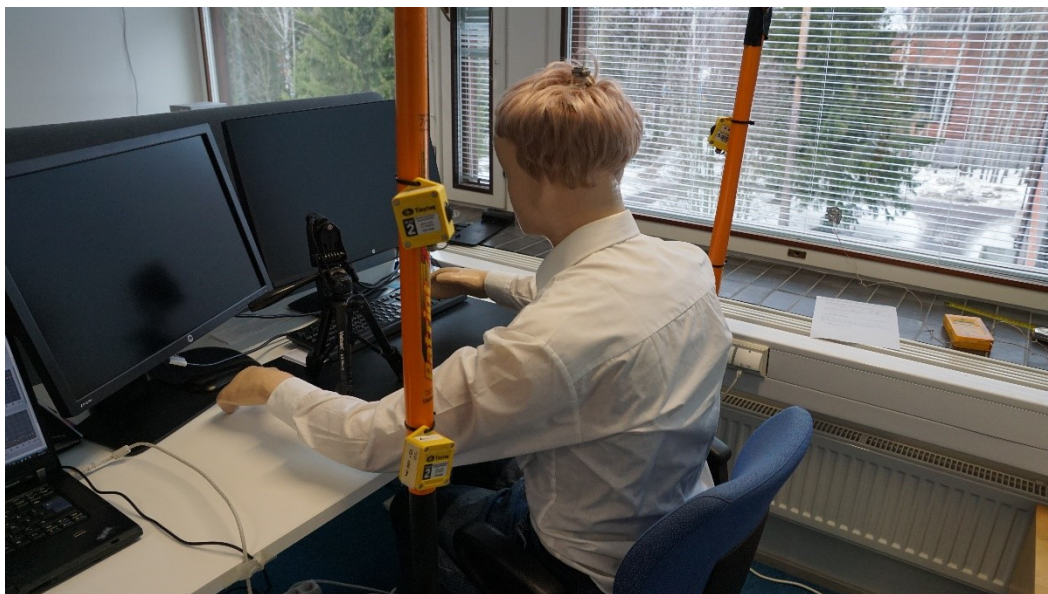
Figure 12. Manikin and temperature measurement rods.
