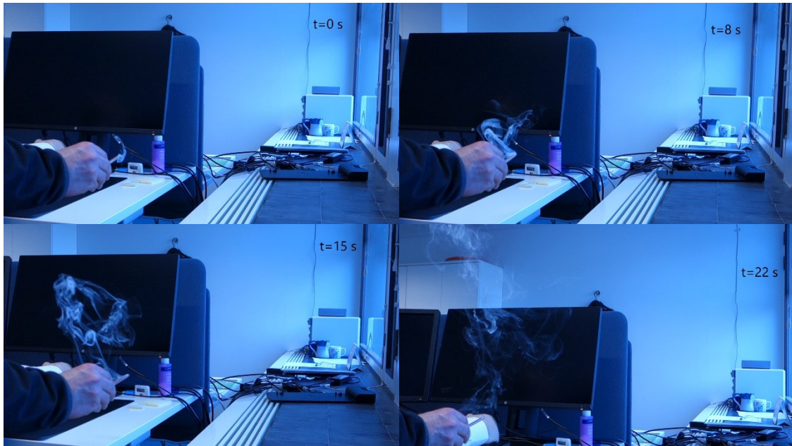
Figure 30. Smoke visualization (case 2) with high thermostat setpoint (23 °C).
