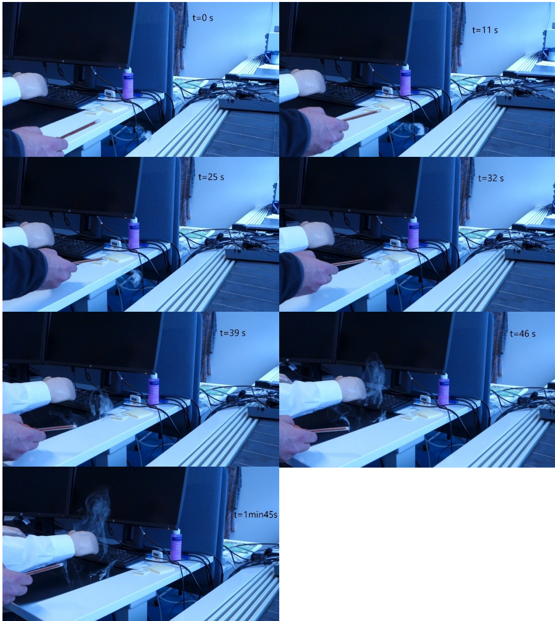
Figure 29. Smoke visualization (case 1) with low thermostat setpoint (19 °C).
