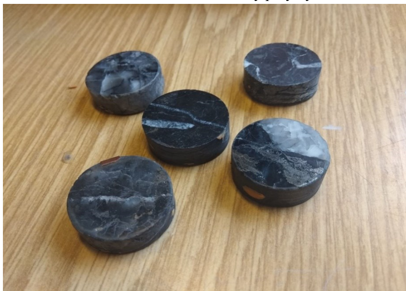
Figure 4-6 Polished core samples according to the Scanning Electron Microscope (SEM) sample specifications.
