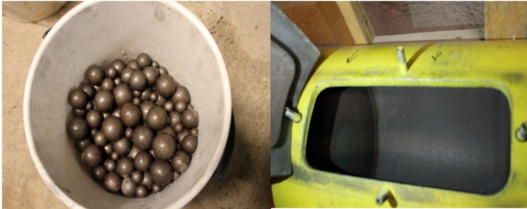
Figure 5-9 Steel ball charge for the bond ball mill
