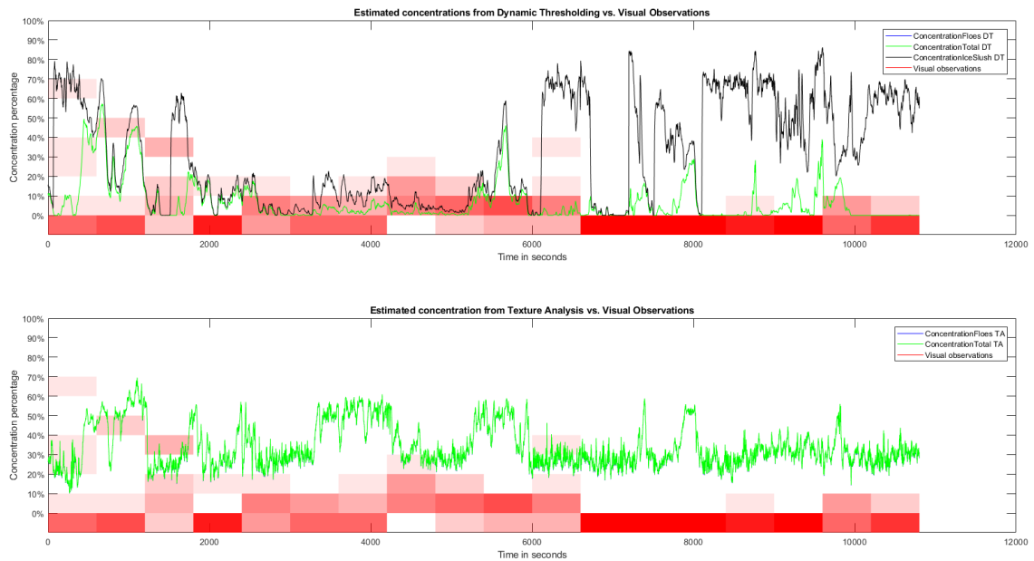
Figure 46. Estimated concentrations vs. visual observations on 5.1.2018 between 14:00-17:00. Blue represents the concentration from the identified and analysed ice floes after post-processing, green is the concentration of the total ice and snow detected in an image, black is the joint concentration between ice and slush and lastly, red is the concentration according to visual observations.
