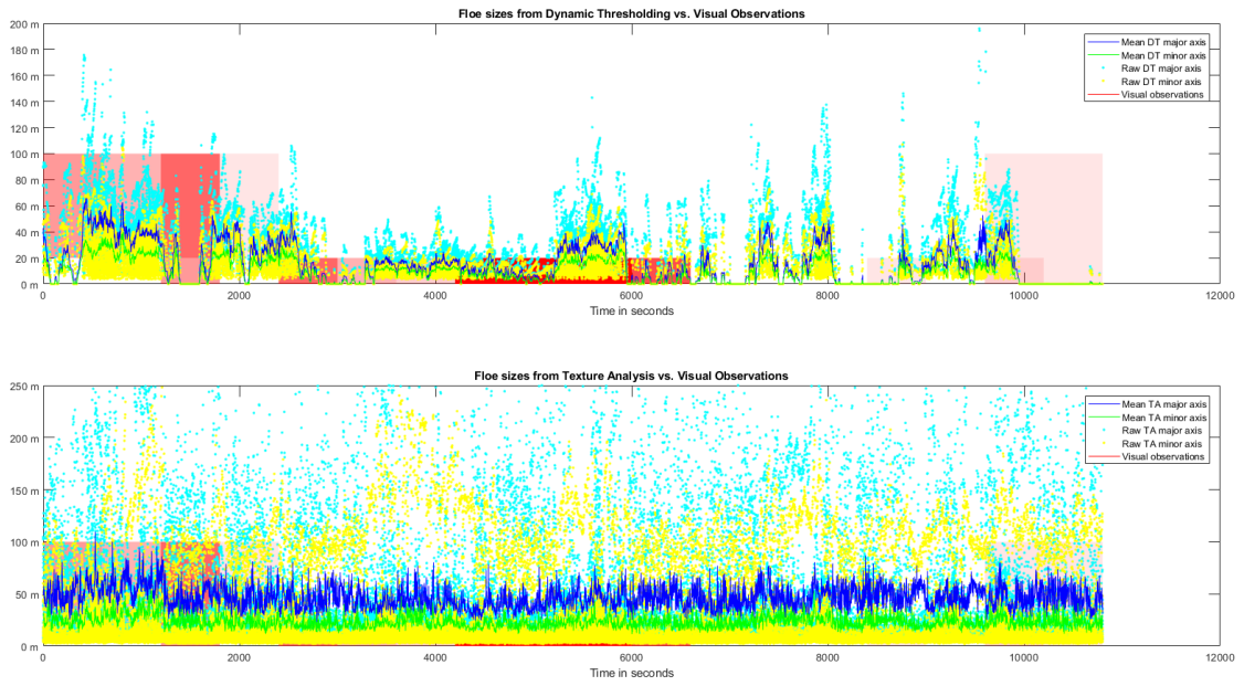
Figure 47. Estimated ice floe dimensions vs. visual observations on 1.5.2018 between 14:00-17:00. Dark blue represents the mean major axis dimension and green the minor axis one for a time instant, while cyan and yellow represent dimensions for major axis and minor axis respectively for individual ice floes and time instants. Red rectangles represent visual observations.
