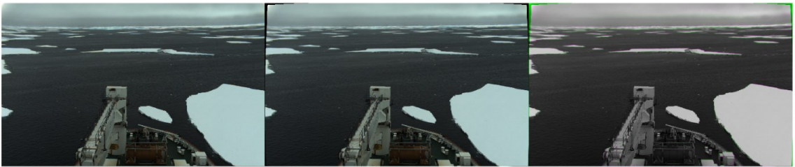
Figure 5. Original image (left), undistorted image (centre) and combination of both images with differences marked in green/pink (right).
