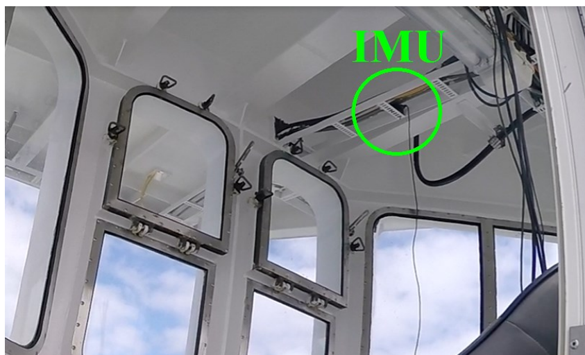
Figure A2. Mounting position of the IMU inside the crow's nest.
