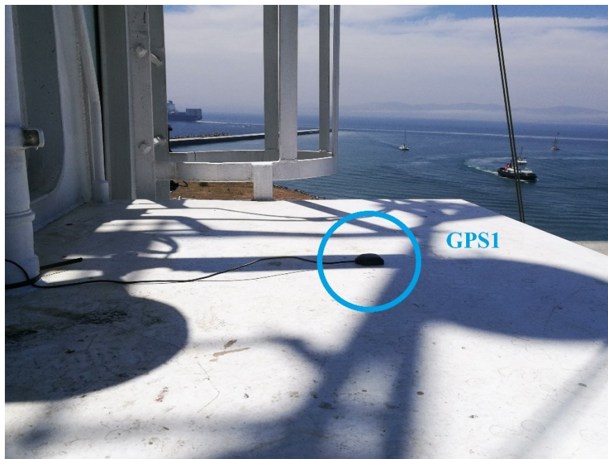
Figure A3. Mounting position of the GPS1 antenna on the S.A. Agulhas II ship.
