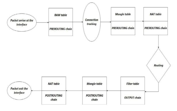
Figure 10: Packets Destined for remote system
