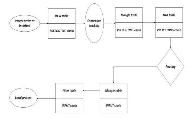
Figure 9: Packets Destined for Local system
