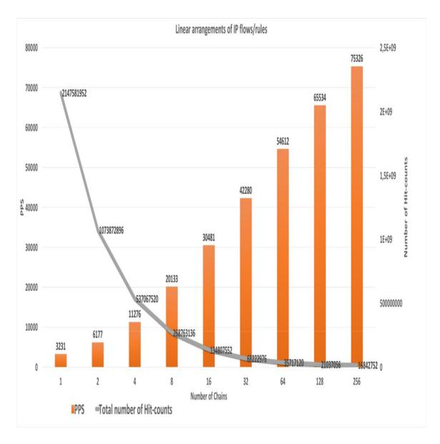
Figure 33: Tcpreplay performance or linear-design of IP flows/rules
