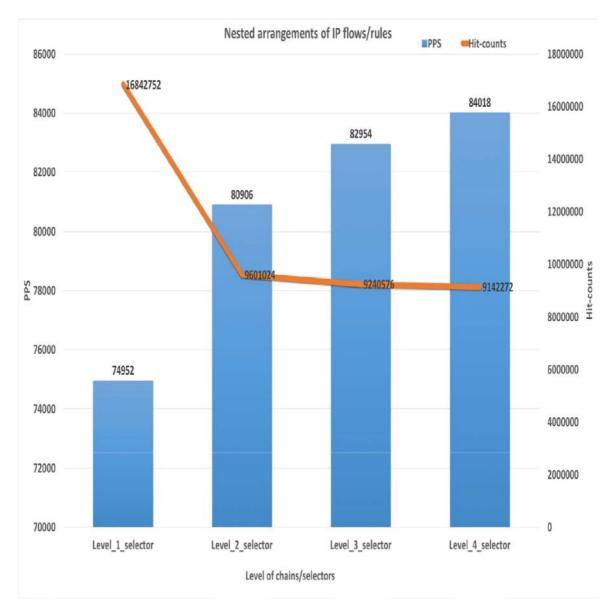
Figure 35: Tcpreplay performance for nested-design of IP flows
