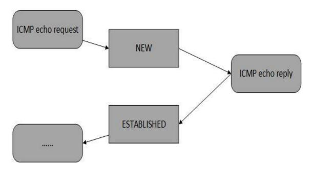
Figure 18: ICMP connections state
