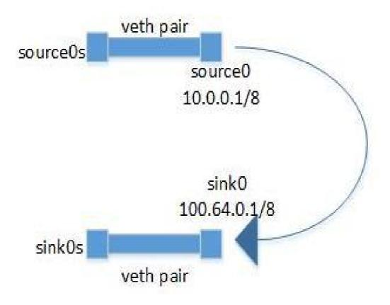
Figure 20: Test Setup for Connection tracking and IP tables
