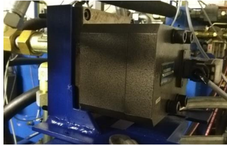
Figure 30. Flow meter Kracht VC 5F1
