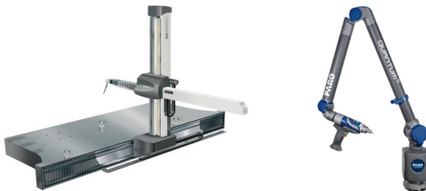
Figure 10. Horizontal arm CMM [22] and articulated arm CMM [25].
