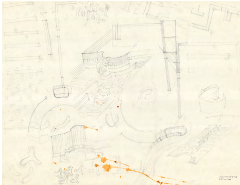
Fig. 86. An undated sketch from the library's design process. In the middle is the curtain dividing the reading and lending halls. (AF)
