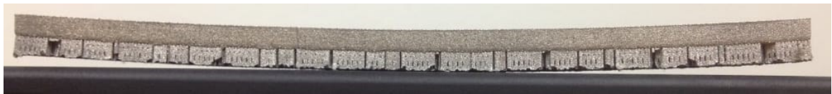
Figure 12: Warping in a 3D printed metal part[15]
