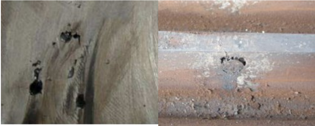
Figure 9: Sand inclusion[21](left) and slag inclusion[21](right)
