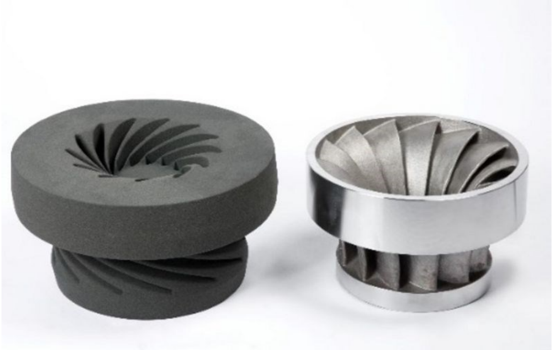
Figure 21: 3D printed sand mould by Voxeljet printer and the casting made from it[30]
