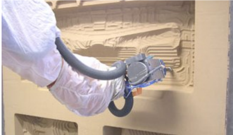
Figure 25: Simtech's robotic milling of sand[35]
