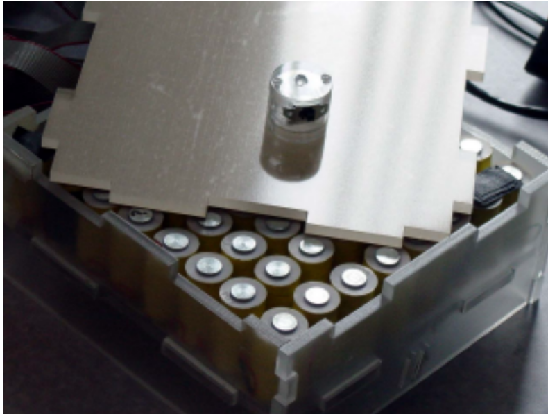
Figure 3.7: Actuated workbench, showing the electromagnet array, by Pangaro et al. [44].
