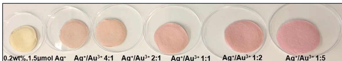
Figure 11. Photography of coated pulp with the combination of AgNPs and AuNPs (Left to right, pure silver ions, with the molar ratios of Ag + /Au 3+ : 4:1, 2:1, 1:1, 1:2, 1:5, the total molar mass is the same for each sample, which is 1.5μmol)
