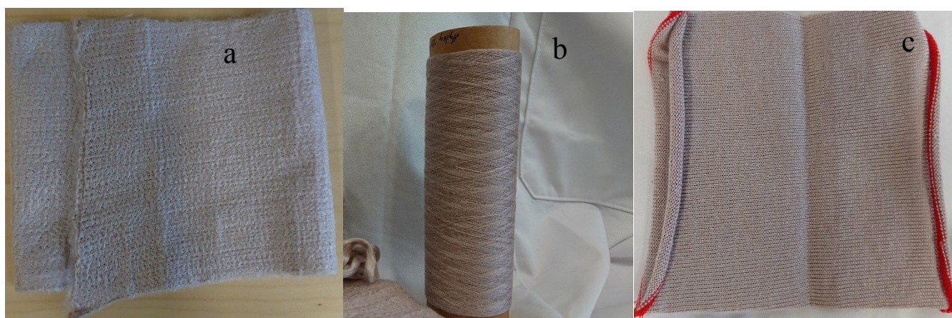
Figure A2. Photography of (a) non-woven sample (b)yarn (c)knitted sample. Produced by AuNPs/AgNPs-pulp, ratio of 1/1
