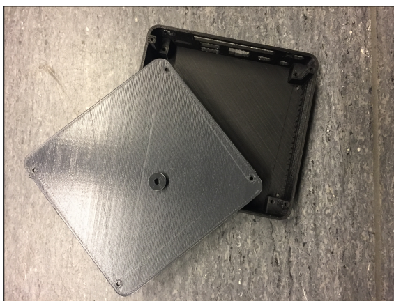
Figure 28: 3D Printed Case for the Intel NUC
