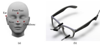
Fig. 2. (a) Approximate infrared sensing locations on face and (b) 3D view of sensing device with four infrared sensors.
