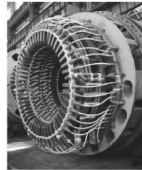
Figure 27 600MW TG stator winding with water-cooled windings [41, p. 21]
