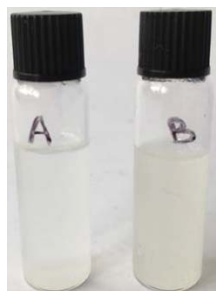
Figure S51. K_4[Fe(CN)_6] (0.0414 M dissolved in H_2O and THF) was added to a solution of ref-PU (0.75 g/mol). The compound was sonicated for 4 hours. After sonication (sample A on the right) and before sonication (sample B on the left) no color change (no Prussian Blue) was observed.
