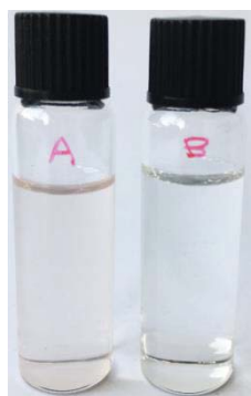
Figure S48. KSCN (dissolved in a 1:1 v/v mixture of MeOH and THF, 0.53 M) was added to the Fc-PMA2 solution, before and after sonication. Fc-PMA2 solutions (2 mg/mL in THF) after 90 minutes of sonication (transparent/pinkish, sample A on the right) and after sonication (transparent solution B on the left). In conclusion the formation of the red complex [\text{Fe}(\text{SCN})_n(\text{H}_2\text{O})_{6-n}]^{(3-n)+} was not observed, excluding the breaking of the ferrocene under ultrasonication.
