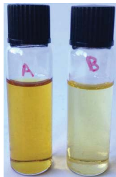
Figure S47. KSCN (dissolved in a 1:1 v/v mixture of MeOH and THF, 0.53 M) was added to the Fc-2 solution, before and after sonication. Fc-2 solutions (2 mg/mL in THF) after 90 minutes of sonication (dark yellow, sample A on the right) and after sonication (pale yellow solution B on the left). Since KSCN interacts only with Fe(III) and not with Fe(II), the darker yellow color of the solution A on the right (after sonication) is probably due to a fragmentation of the polymer in smaller parts that could interact with KSCN. In conclusion the formation of the red complex [\text{Fe}(\text{SCN})_n(\text{H}_2\text{O})_{6-n}]^{(3-n)+} was not observed, excluding the breaking of the ferrocene under ultrasonication.
