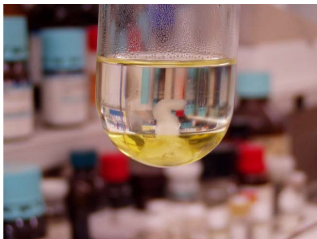
Figure 114. Picture of polyethylene in a yellow solution of Ni(II) catalyst.
