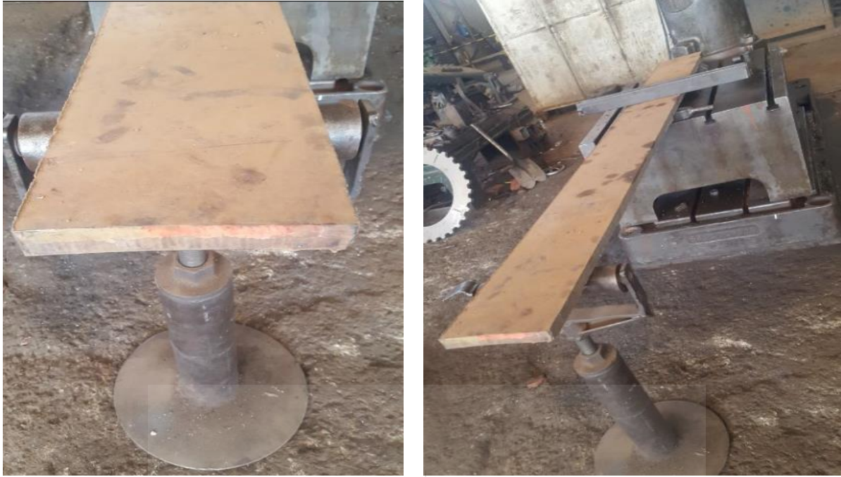
Figure 4.12: The steel bar mounted on the drilling machine
