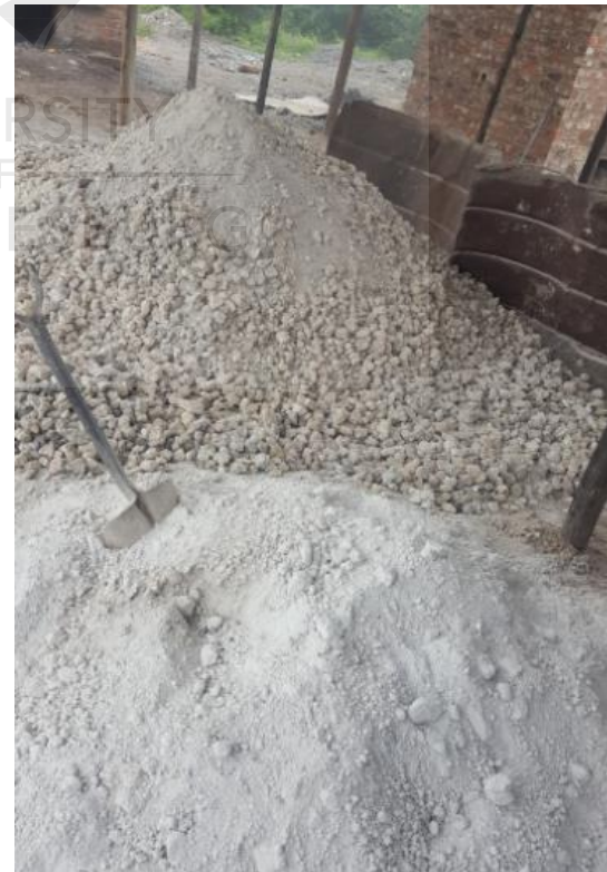
Figure 5.4: Quicklime changes to white powder when water is added to it.
