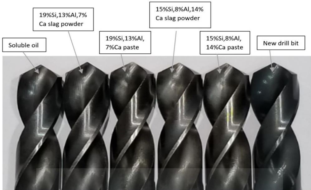
Figure 4.19: Used drill bits at close range being compared to a brand new one
