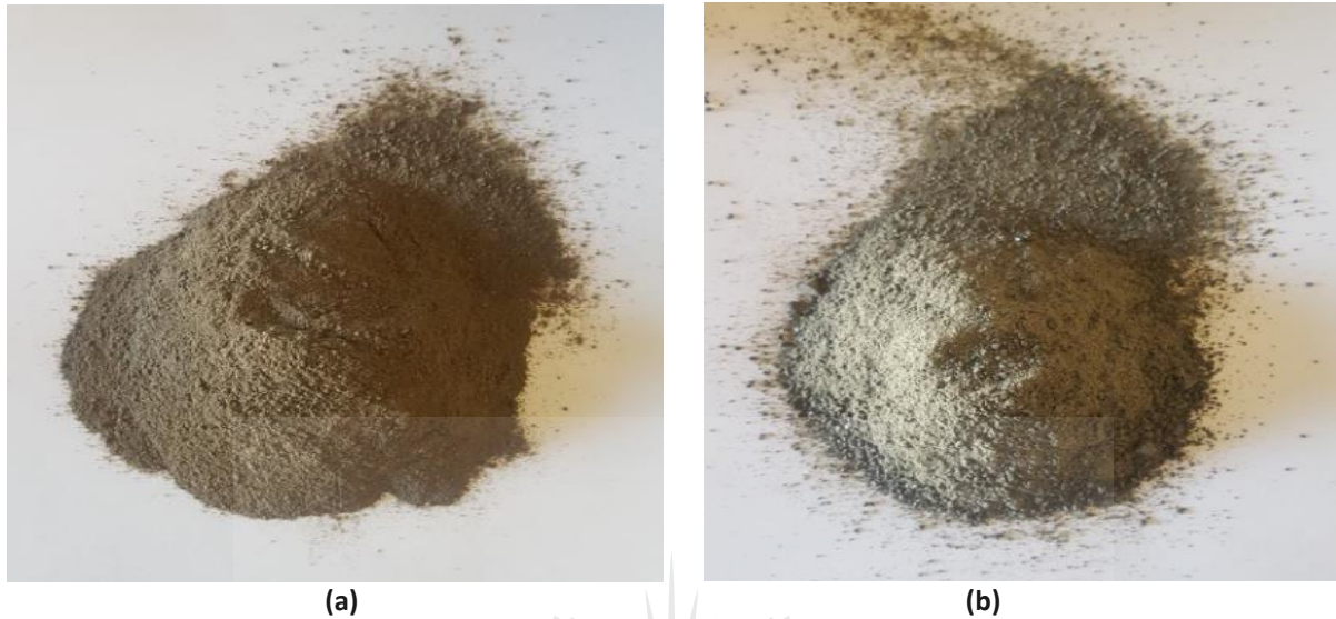
Figure 4.7: Slag samples ground into powder (a) 15%Si,14%Ca,8%Al slag (b) 19%Si,7%Ca,13%Al slag
