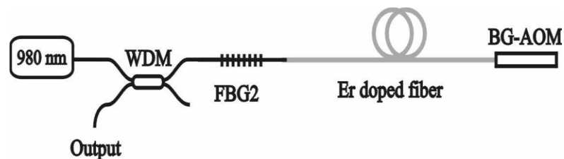
Figure 2.14: All-fiber Q-switched laser using an acousto-optic modulator of a fiber Bragg grating linear cavity (Delgado-Pinar M. et al., 2006).
