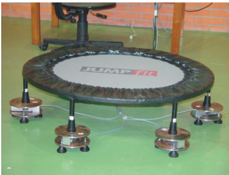
Figure 1. Rebound exercise mini-trampoline with attached load cells
