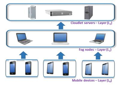
Figure 2. Classical three-tier MEC architecture.
