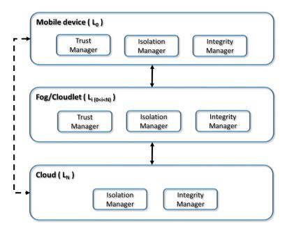
Figure 3. System architecture for a multi-tier MEC paradigm deployment.
