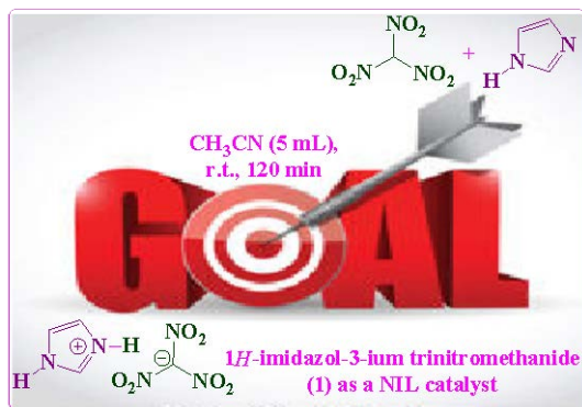
Scheme 1. Synthesis of 1 H -imidazol-3-ium trinitromethanide catalyst (1) {[HIMI]C(NO 2 ) 3 }.
