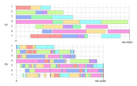
**Fig. 2.** Gantt charts representing the obtained schedules for instance P5.1 S1, when (a) lot streaming is forbidden, and when (b) lot streaming is allowed. There are 8 lots to be manufactured in a shop with 7 machines. Each lot (with different colors) requires 4 operations, each of which can be processed in a set of 2 or 3 alternative machines.
