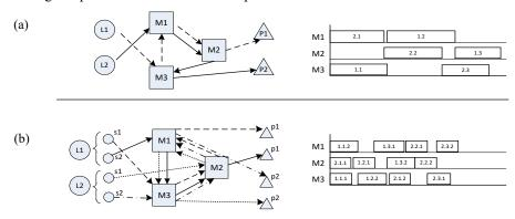
Fig. 1. (a) An FJS processing two lots without lot splitting. (b) Same FJS processing two lots with lot streaming.
