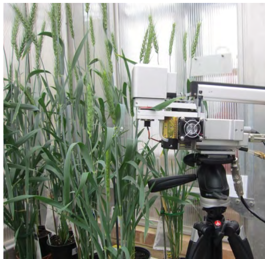
Figure 1. Gas-exchange analyses (LI-6400XT) of wheat T1 transformant plants growing in the glasshouse.
