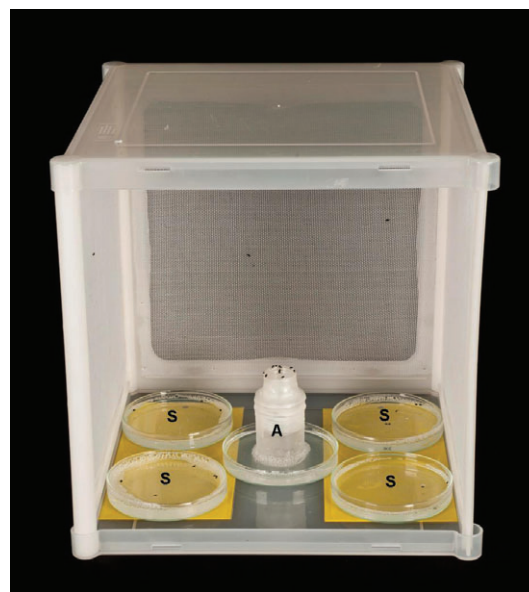
Figure 1. Insect flight cage ('Bugdorm-1', www.megaview.com.tw ) with the front removed to demonstrate the experimental set-up for the flight bioassay. (A) The central release point, consisting of the release vial containing ca 50 pollen beetles at the start of the run, the ice jacket around the release vial and the central water trap to prevent beetle escape by walking. (S) Four 'sink' water traps to reduce the chance that pollen beetles that escaped the central release point would return to the central water trap.
