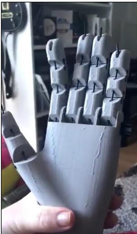
Figure 6.2: Prosthetic hand built by Group 2 participant
