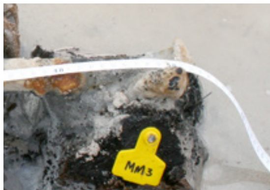
Figure 30: Plastic tag used to mark sampling areas on wreck.
