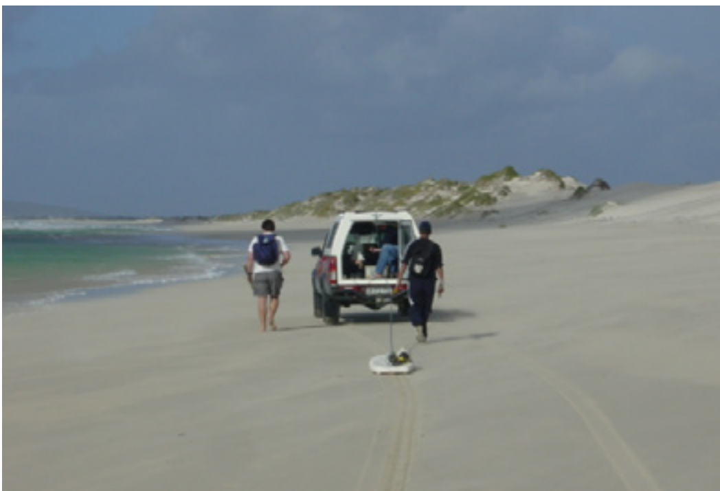
Figure 10: Magnetometer being towed behind a vehicle on a surfboard.
