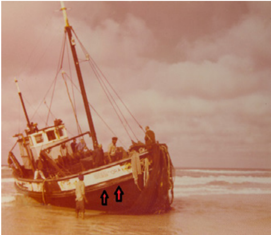
Figure 49: Wreck of the fishing trawler Dora K. (red arrows indicate rubbing strake on the vessel.)
