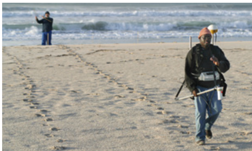
Figure 17: Handheld magnetometer survey with the assistance of Anglo American.
