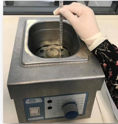
Figure 4: Water bath post-polymerization group
