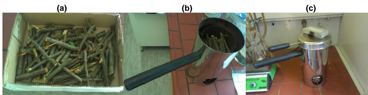
Figure A.1. Preparation of the biochar – (a) Dry 10 cm long branches, (b) pyrolysis oven with branches placed horizontally, (c) pyrolysis process.
