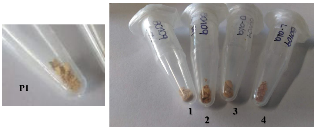
Figure 2.14. Solids of P1 before and after insertion of guest molecules: 1) D-phenylalanine; 2) L-phenylalanine; 3) D-alanine; 4) L-alanine.
