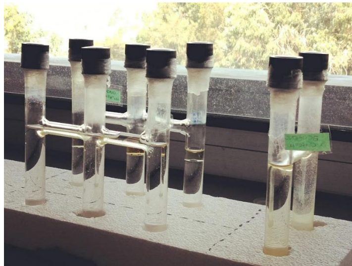
Figure 2.4. H-shaped tubes used in the synthesis by slow diffusion.
