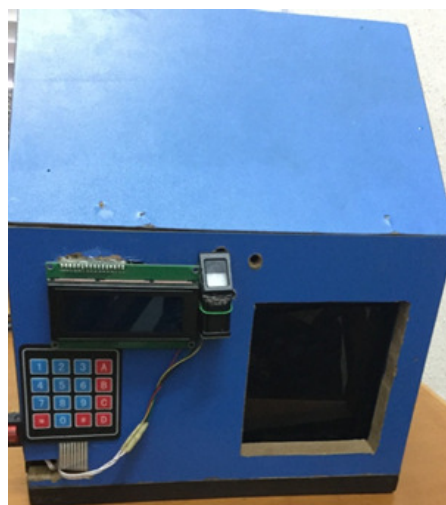
Figure 3 The Bank Vault Access System's Hardware
