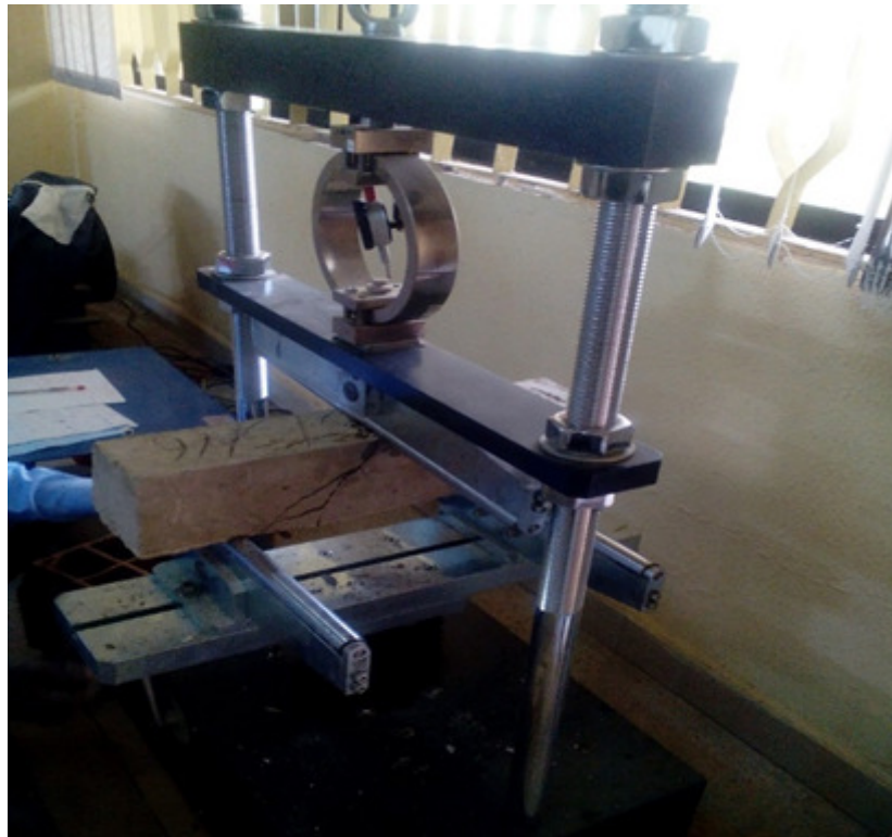
Plate 1 Flexural machine and flexural beam under load
