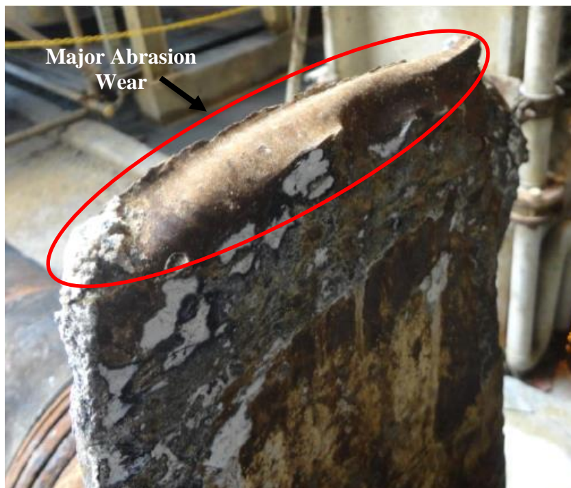
Figure 1: Blade Condition after 6 Month of Process.
