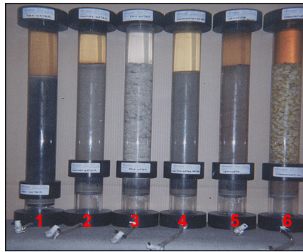
Fig. 5. Long-term Test Cells of Prehydrated GCL when permeated with non-standard liquids. (1) Mine Water, (2) Contaminated Water, (3) Rain water with Limestone Chip, (4) Sea Water, (5) Synthetic Leachate, (6) Transformer Oil
