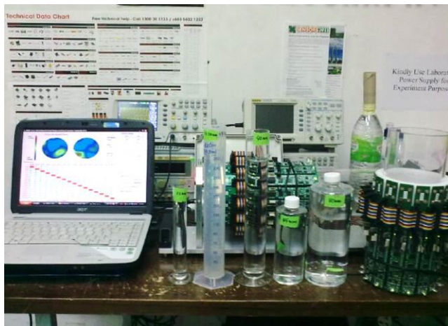
Figure 5 Portable segmented ECT with bottle and test tube used to create phantoms inside the ECT sensor. The bottle and test tube were filled with water, creating a phantom of annular water flow
