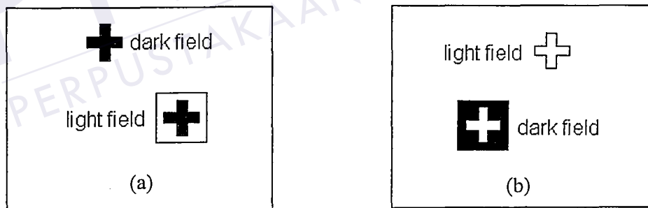
Figure 2.2: Alignment mark design. (a) Alignment mark for mask 1; (b) alignment mark for mask 2, mask 3 and mask 4.
