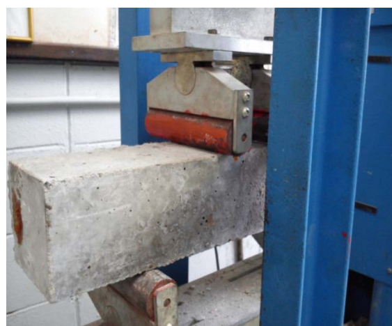
Figure 7 Flexural test set up
