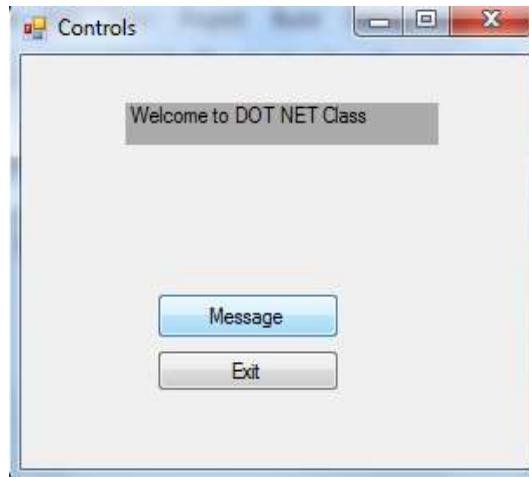
Figure 3.13: Click on the Message Button and “Welcome to DOT NET Class” appears in the Label
