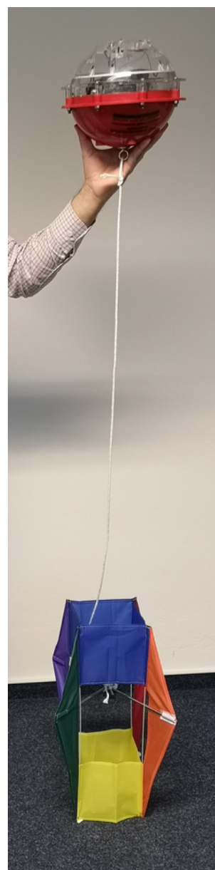
Figure 2: Drifters ODi used during the experiment. The drifter sails were mounted 1.5 m under the sea surface.
