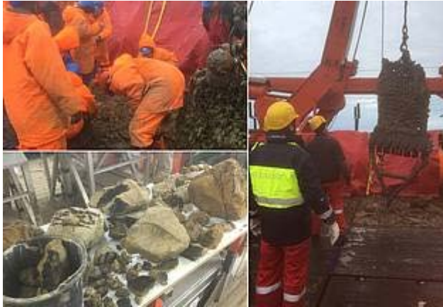
Fig. 2: The stone dredge is onboard (right picture), mud and stones are identified and cleaned (upper left), and then presented on a table in the wet lab (lower left). (Photo: R. Stein/AWI)
