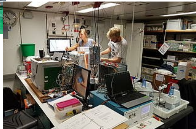
Pic. 4: We managed to fit three gas chromatographs on this table. They will measure climate active gases from water samples. (Photo: W.-J. von Appen)
