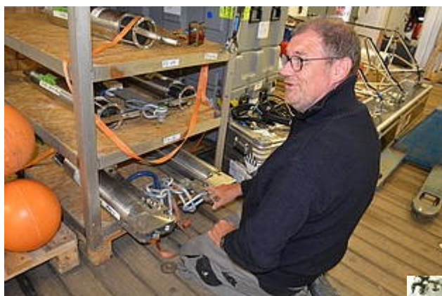
Pic. 1: An acoustic release, which is mounted at the bottom of a mooring line, is being tested. The release allows us to unfasten the mooring from the sea floor after 1 to 2 years in the water and to retrieve it at the sea surface. (Photo: J. Vernaleken)
