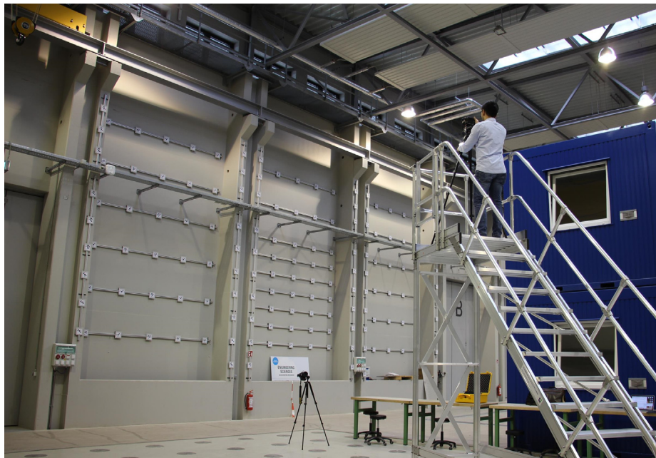
Fig. 5. Process of camera calibration using a large scale calibration wall with the dimension of about 13,0 × 7,0 m and 163 targets.
