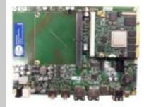
Q7 carrier board 2 x Cortex-A9 2 GFLOPS 1 GbE + 100 MbE 7 Watts 0.3 GFLOPS / W
