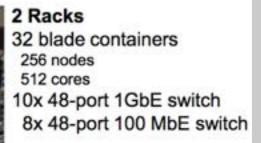
512 GFLOPS 3.4 Kwatt 0.15 GFLOPS / W
