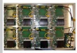
**1U Rackable blade** 8 nodes 16 GFLOPS 65 Watts 0.25 GFLOPS / W
