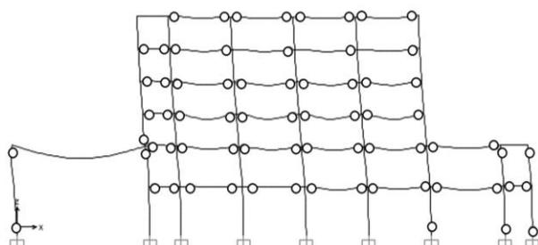
**Figure 8.** Frame 1 Plastic Hinges due to Design Earthquake in x-direction
