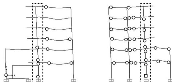
**Figure 9.** Frame 6 Plastic Hinges due to Design Earthquake in x-direction
