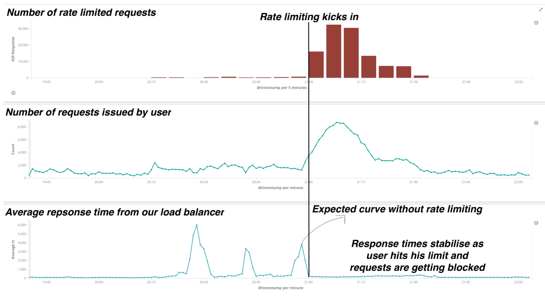
Figure 7.4: As rate limiting kicks in, average response times starts to stabilise as number of requests passed through the filter decreases.
