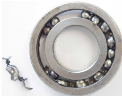
Figure 4.7.: Bearing failure due to cage damage
