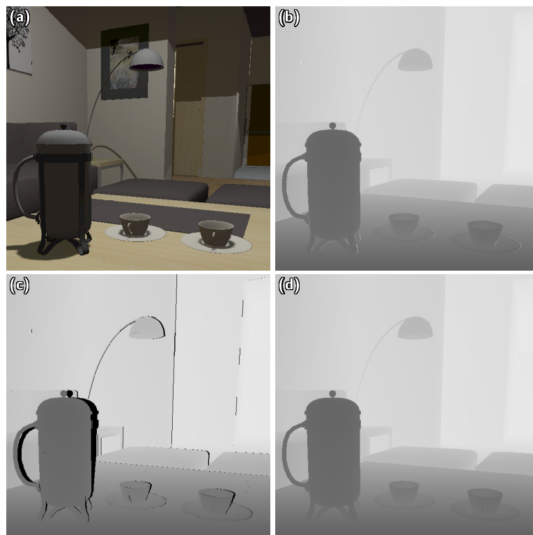
Figure C.1: A comparison of depth reconstruction quality. (a) A new view synthesized with our method (using two depth-layers). The full-image took 6.5ms to render. The synthesized depth for (b) two-layer and a (c) single-layer configuration. (d) The reference was generated with NVIDIA OptiX in about 20ms. In both cases we report combined construction and tracing times.
