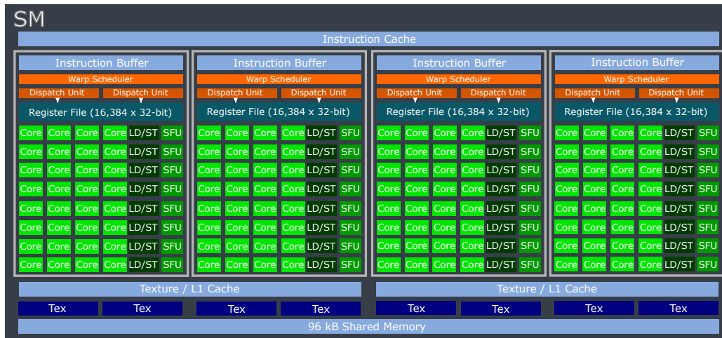
Figure 3.1: The diagram in this figure shows all components of a Streaming Multiprocessor (SM) of the GP104 architecture [NVIDIA, 2016](redrawn after [NVIDIA, 2016]).
