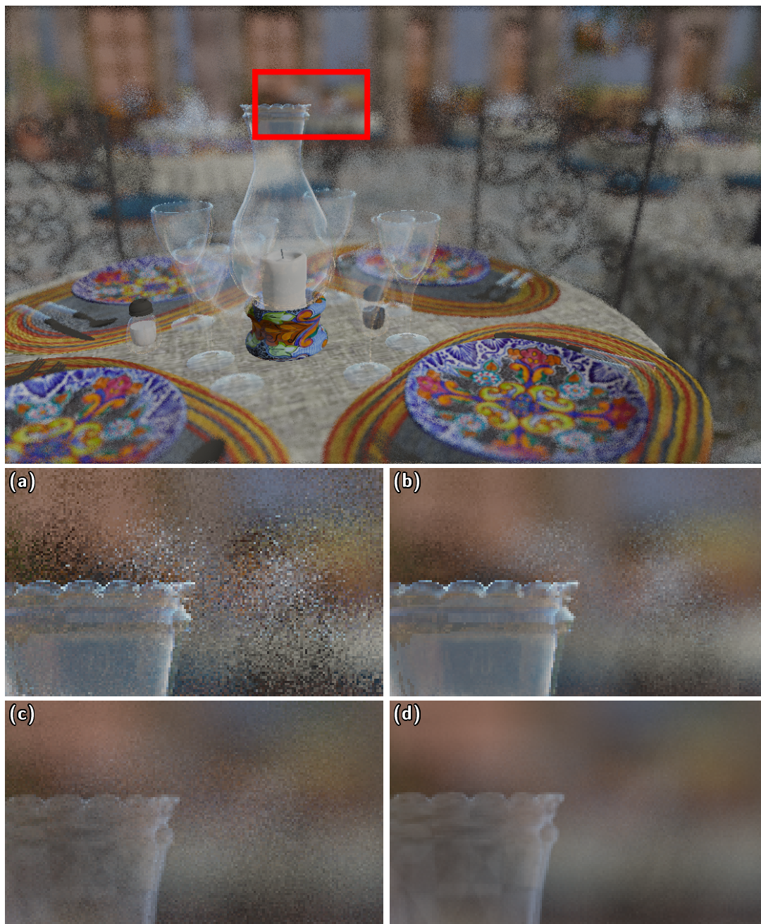
Figure 8.16: Quality comparison of our approach (a) using 4 Dof samples times 8 motion samples with time sampled ray tracing (b) using 32 samples. Differences of the Blender references (c) 32spp and (d) 256spp) to our approach are due to proper 5D sampling. Cycles jitters lens as well as time samples. The reference images were rendered in 2.0 and 14.5 minutes respectively.
