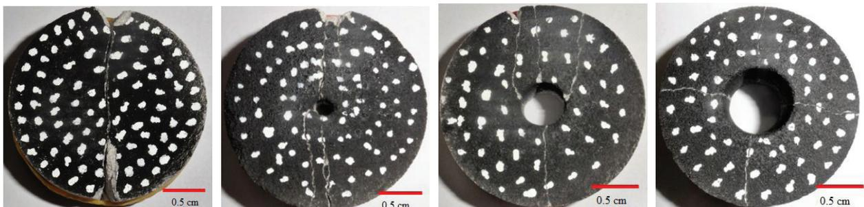
FIGURE 2. Mode of failure in a) solid, b) 0.1, c) 0.2 and d) 0.3 diameter ratio in ring disk under Brazilian test
