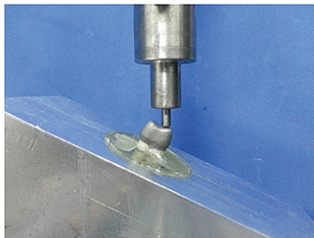
Fig. 1. The position of a specimen in a customized metal holder in a universal testing machine for static loading at 25°
